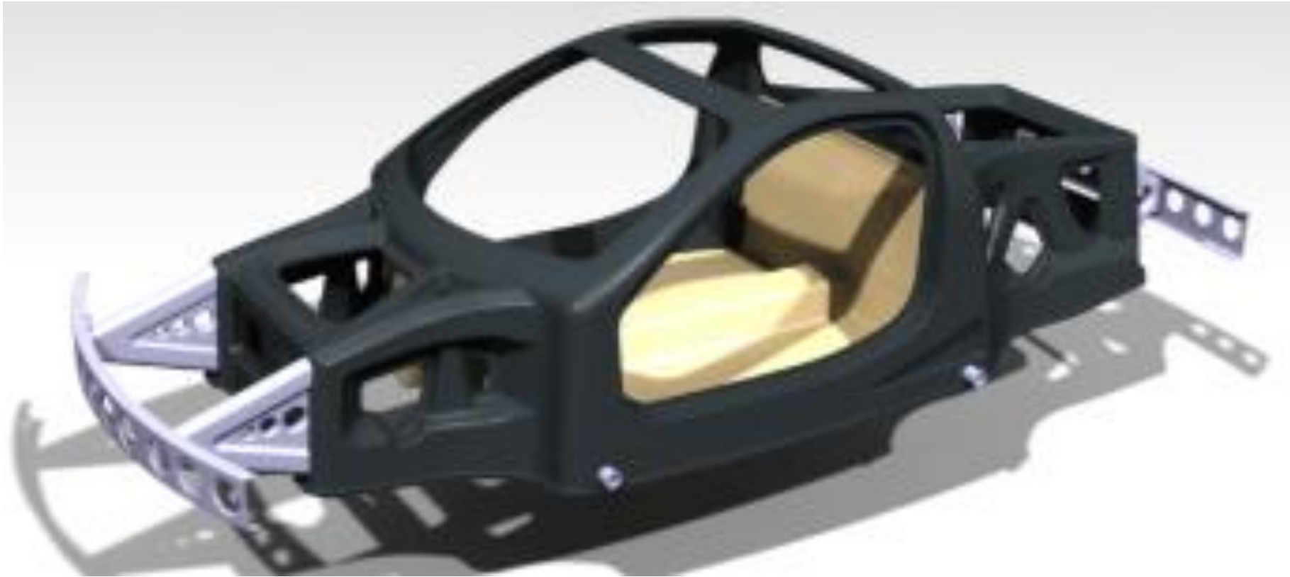
Carbon Body with aluminum front and rear crash system
